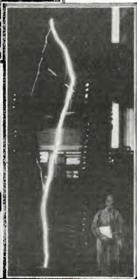
Below we see 3,000,000-volt artificial lightning stroke produced in G. E. Laboratory at Pittsfield, Mass. Note man.
