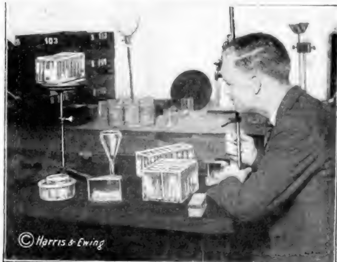
The engineer shown in the photograph above is demonstrating the use of the Strain Detector in testing storage battery cells.
