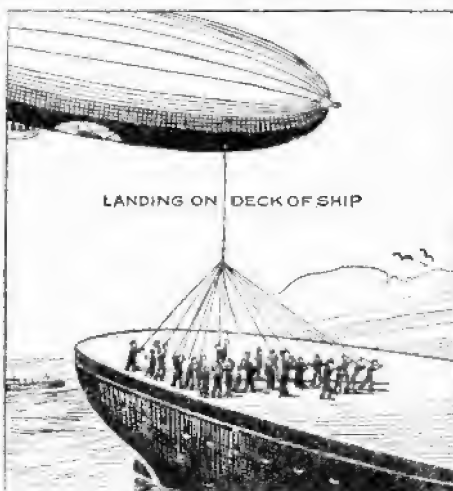
When landing upon the deck of a ship, a number of ropes are employed as shown here.
